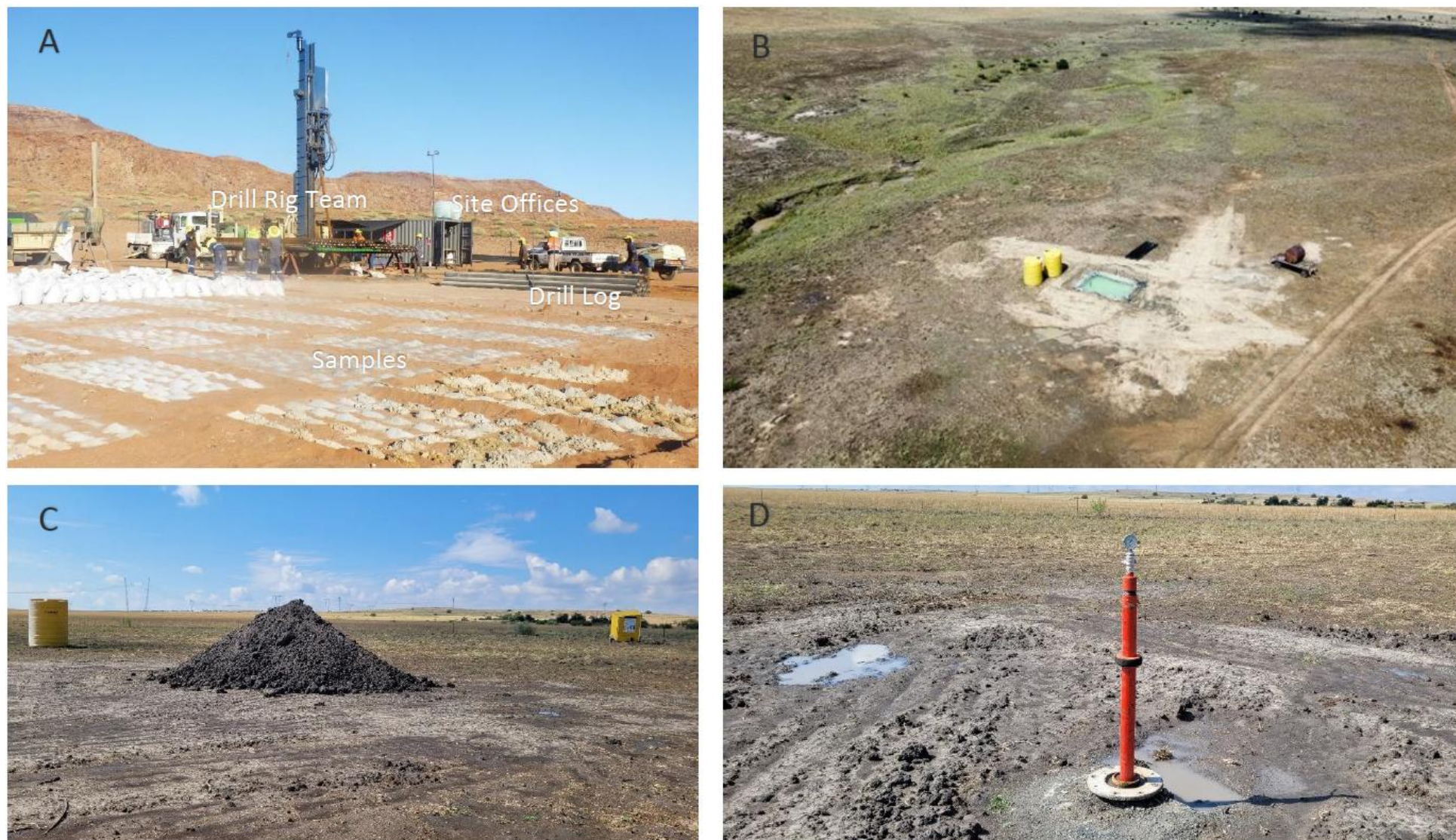
Figure 2: Exploration drilling and potential impacts. (A) Showing the drilling process and associated infrastructure, (B) Showing the drill pad footprint at one of the active Motuoane drilling sites, (C) Showing some of impacts associated with drilling activities.
